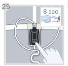
Press the power button again for about 8 sec. until the device vibrates and the LEDs start blinking blue.
