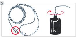
Attach the cannula to Respiro and rotate the connector slightly clockwise until you feel it connect.
