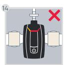
If any LED indicator blinks **red** or **yellow**, check that the item corresponding to the indicator is connected properly. Explanations for the indicators can be found on the **next page**.
