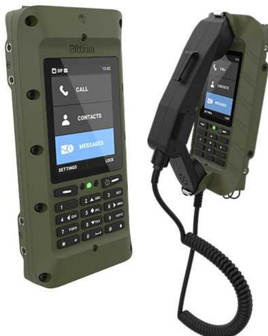
Meanwhile, in April, the company launched the Tough VoIP Field Phone 2, an upgraded variant of its predecessor, which can be used for tactical IP-based communications.
