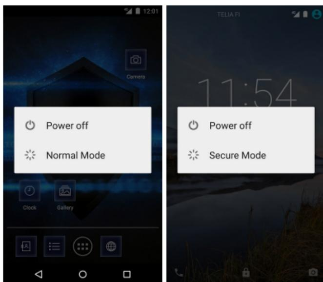
Pressing the power key lightly on top of the device opens the Power key menu with options for Power off, Normal Mode and Secure Mode, depending on the currently active mode.
