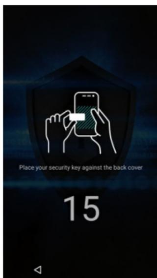
If unlocking fails or the timer runs out, the device remains locked. A PIN code is required again before using the Security Key to unlock the device.
