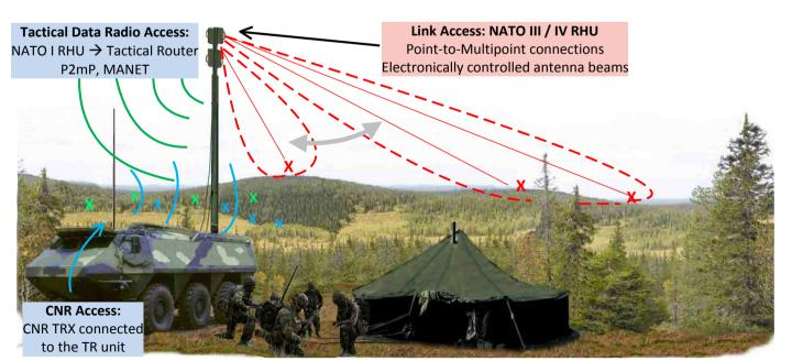
Figure 4: An example of the connectivity provided by a single EB TAC WIN node equipped with two Radio Head Units and an interface to a legacy CNR system. (*Copyright Elektrobit*)
