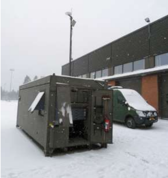
1521988 - Exterior view of CBRN-protected Command Post (CP) Module A being tested as part of the M18 C3 system. CP Module A has workspace for up to five operators. (IHS/Peter Felstead)
