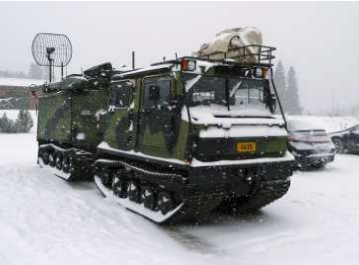
1521992 - Exterior view of M18 Communications Vehicle A all-terrain module. Clearly visible is the Band I/Band III antennas, as well as a stowed mast for Band III/IV point-to-point and point-to-multipoint transmissions (without the antennas fitted). (IHS/Peter Felstead)
