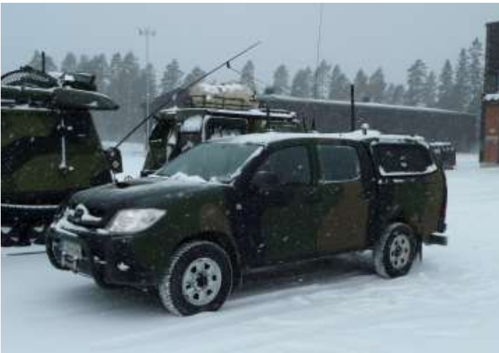
1521994 - Exterior view of the M18 Communications Vehicle E showing the VHF, Band I, and GPS antennas. Currently the Toyota Hilux platform is used for testing purposes. (IHS/Peter Felstead)
