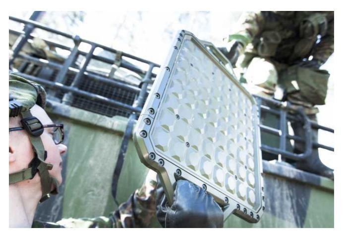
TAC WIN is a modular system that supports Mobile Ad Hoc Network (MANET), Point-to-Multipoint, and Point-to-Point networks, optimised to create and maintain maximum levels of command and control, situational awareness and information security, no matter where or when troops are operating.
