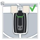
The LEDs are lit in **green** to indicate a successful recording start
