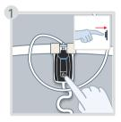
You can shortly press the power button to mark times when you are not sleeping, such as going to bed, going to the bathroom, waking up... (Optional)
