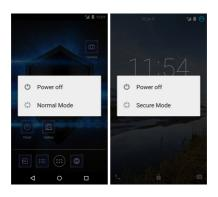
Pressing the power key lightly on top of the device opens the Power key menu with options for Power off, Normal Mode and Secure Mode, depending on the currently active mode.
