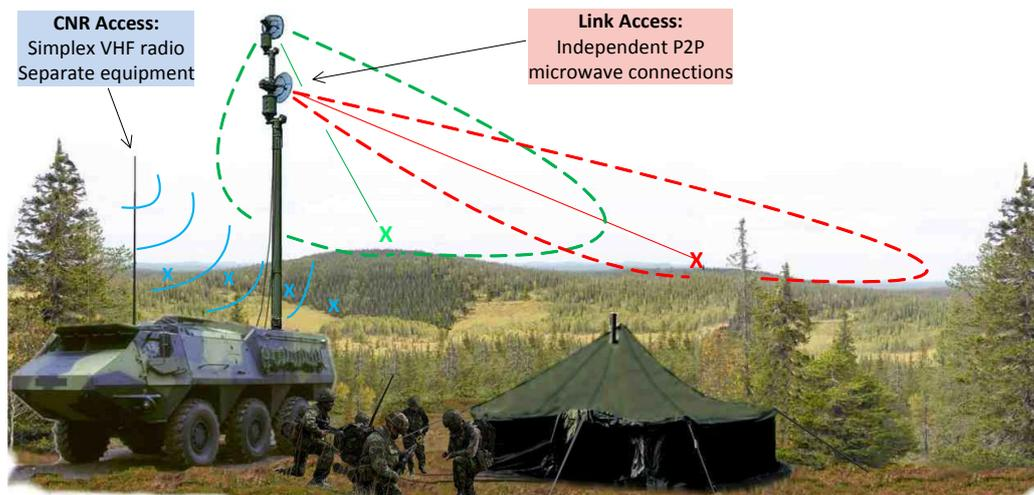
Figure 2: The conventional point-to-point link solution (Copyright Elektrobit)
