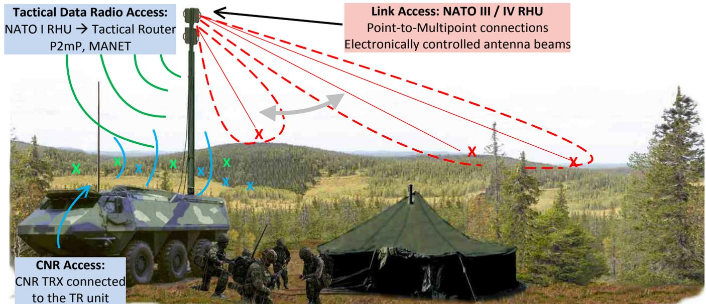
Figure 4: An example of the connectivity provided by a single EB TAC WIN node equipped with two Radio Head Units and an interface to a legacy CNR system. (Copyright Elektrobit)
