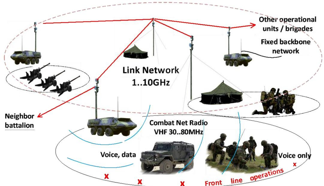
Figure 1: Tactical communications system architecture example (Copyright Elektrobit)
